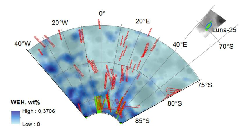
Figure 1 – Map of WEH abundance in the South polar region (Sanin et. al., 2017) and possible stereo coverage of LROC NAC images
